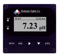
Automatic and manual temperature compensation: Due to the dependence of pH value and electrical conductivity on temperature, very accurate temperature compensation is possible in a wider temperature range than the analog method.
